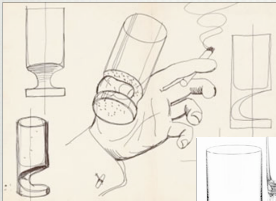
SMOKE GLASS. Smoking and drinking with one hand. The other hand is left free to gesticulate while talking. Design by Joe Colombo.
