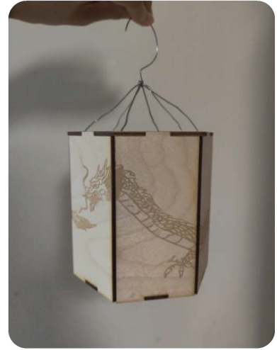
Testing laser cutting file and etching of dragon. Experimented with method of connecting all the parts
