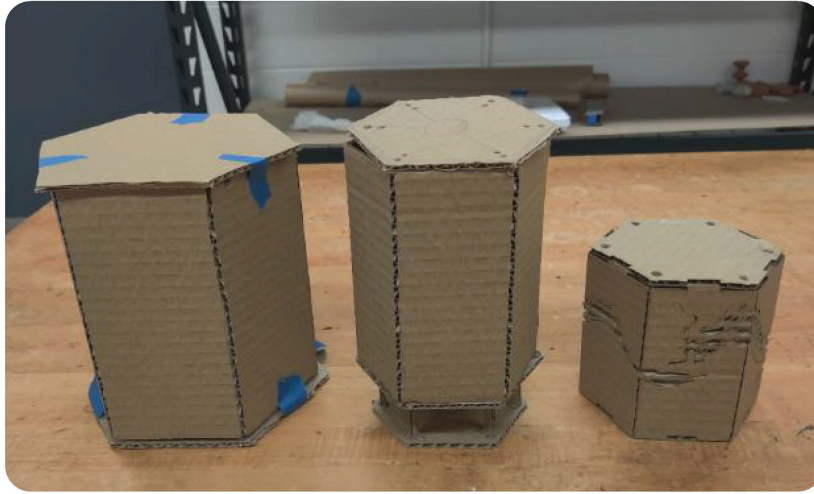
Cardboard models to test overall size and form. Experimented with the hexagonal pieces sitting flush to one another or touching at the edges. Was originally a standing lamp but became a hanging lantern through the iterative models.
