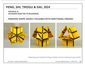
Feng and Shi conducted a longer kinematic analysis and determined that the shape is rigidly foldable if additional creases are placed on the diagonals of some of the square plates, thus admitting only rigid pates and rotational hinges.
