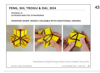
The auxetic property of the modified shape is demonstrated in this folding sequence. A detailed technical report on this new metamaterial has been accepted and will presented at the 6th International Conference on Reconfigurable Mechanisms and Robots (ReMAR 2024) which will take place in Chicago in July of this year.
