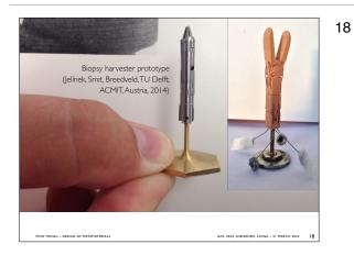
The sea urchin model has inspired new instrumentation, like this prototype of a biopsy harvester developed at Delft university of Technology, which mimics, in reverse, the opening and cutting motion of the teeth.
