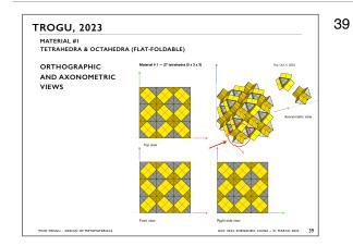
Compared to the previous view, the material is here seen lying on the extrusion sides instead of lying on the faces normal to the extrusion, allowing to construct a cubic patch of 3 x 3 x 3 tetrahedral unit cells.
