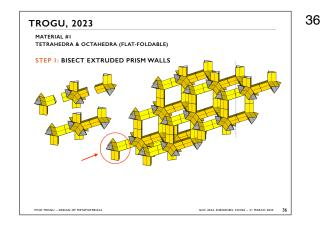
We apply the bisection to the walls of the extruded prisms, so each prism will now have six creases instead of three.
