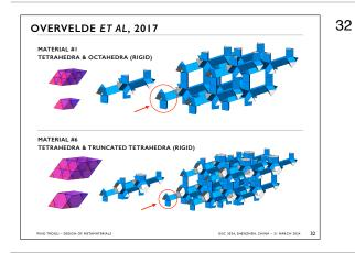
... with all the 28 materials that were examined. Materials #1 and #6 were rigid owing to the rigidity of the triangular prisms in the extruded tetrahedrons.
