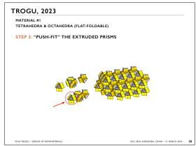
We "push-fit" the extrusion pairs to increase the density of the material.
