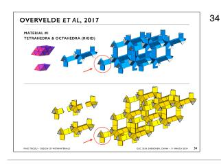
Without bisections, this material is also quite "open" on account of the double extrusion lengths and the larger octahedra which form when tetrahedrons are assembled together.
