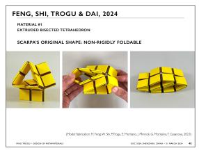
Recently, a kinematic analysis was conducted by Feng and Shi on the original tetrahedral unit, and it was determined that while the shape is flat-foldable, this is possible because of deformation of the creases.
