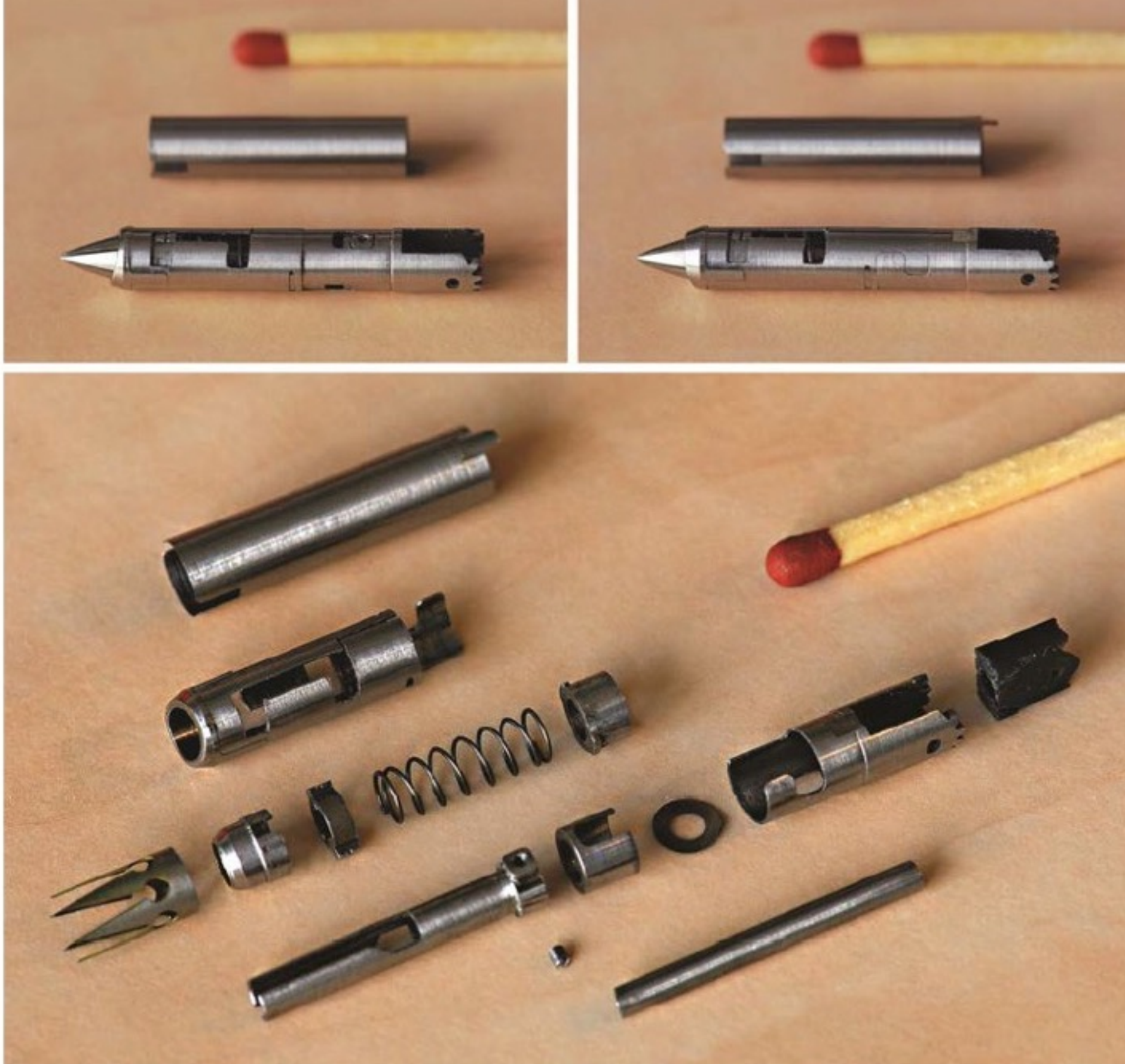
Figure 9.4 Final manufactured steerable opto-mechanical biopsy harvester prototype.
