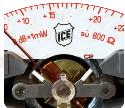
Above: Inside view of a voltmeter's wrapped coil and analog needle. Left: Analog voltmeter that reads amperes.
